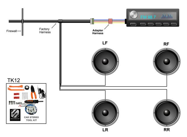
If you are just looking to improve your sound quality and the OE head unit is still working, consider replacing the OE factory speakers as a first step in your upgrade. The inexpensive speakers installed in most vehicles deteriorate with age. You will be amazed at the improved sound you get from higher quality aftermarket speakers.
