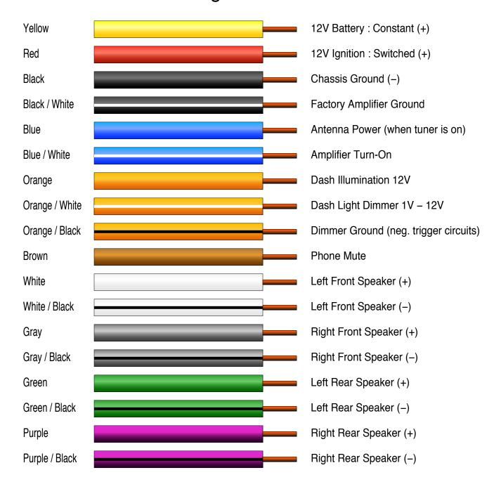
The color codes used on aftermarket car stereo connector harness's conform to the E.I.A (Electronics Industry Association) standards. These colors often differ from the wiring colors used by vehicle manufacturers. Always refer to your stereo owner's manual for specific wiring details before making any connections.
