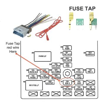
The long external red wire provided is to tap into an accessory position wire or fuse tap. You're looking for a wire/fuse that is switched "on" and "off" with the key.
